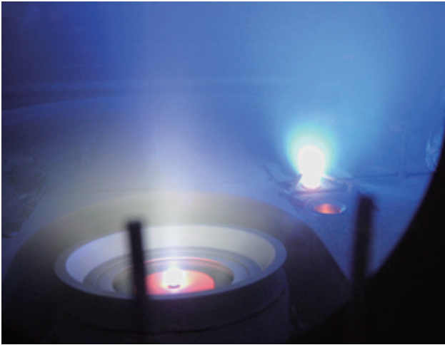
Discharge above the crucible and plasma source during ITO film deposition
